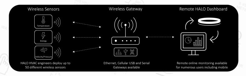
Our wireless sensors and secure internet gateways notify you about abnormal HVAC events, energy use and temperatures, system degradation, humidity, air pollutants, air pressure, water, vibration, velocity, motion, security & much more. We tell you the exact energy consumption in kWh of each individual component of your HVAC system, in real time or over a period, remotely.
